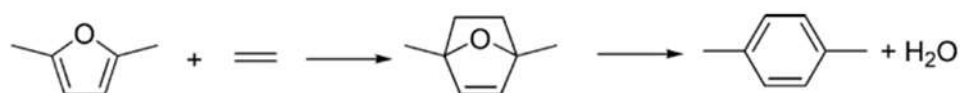
Figure 5. Production of p -xylene via Diels–Alder cycloaddition with ethylene and subsequent dehydration.
