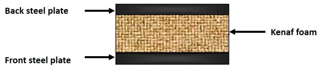
Figure 12. Cross sectional of sandwich armor plate with kenaf foam.
