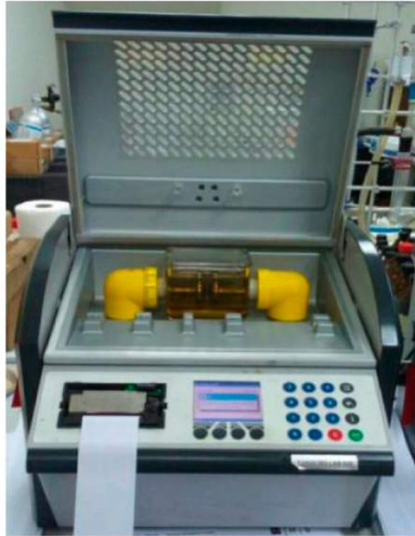
Figure 3. Oil test set.
