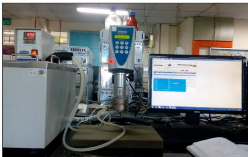
Figure 15. Brookfield DV-II + Pro Automated viscometer with CP-41 spindle.
