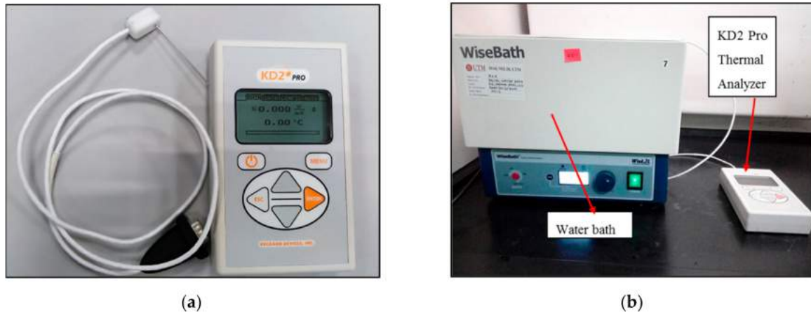
Figure 17. Thermal conductivity instruments: (a) Thermal Properties Analyzer, Decagon KD2-Pro Conductivity meter with KS-1 sensor, (b) Wise water bath used to conduct thermal conductivity test.
