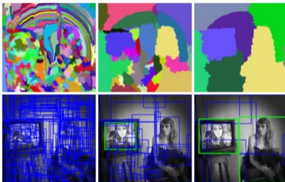
Figure 9: Selective search applications of the algorithm with the visualization of the (top) segmentation and (bottom) region proposals [54].
