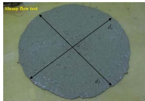
Figure 5. Slump flow test for measuring the filling ability of SCGCs.
