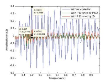
**Figure 16.** PID controller tuned by ZN and PSO methods for vibration suppression in time domain using multiple real disturbance. PID: proportional-integral-derivative; ZN: Ziegler-Nichols; PSO: particle swarm optimization.
