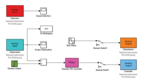
**Figure 21.** Block diagram of PID-based controller using MATLAB/Simulink. PID: proportional-integral-derivative.
