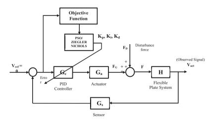
**Figure 9.** The block diagram of PID-based controller tuned by Ziegler–Nichols and particle swarm optimization methods. PSO: particle swarm optimization; PID: proportional–integral–derivative.
