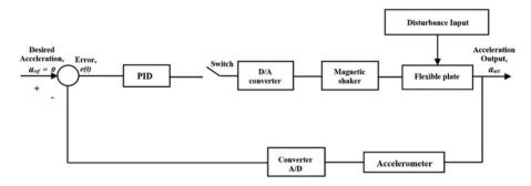
**Figure 20.** The schematic diagram of the controller used in the experiment. PID: proportional—integral—derivative.
