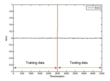
Figure 6. Error between actual and estimated output of the system using PSO modeling.
