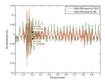
**Figure 18.** Comparison in time domain between PID-ZN controller and PID-ABC controller with multiple real disturbance. PID: proportional–integral–derivative; ZN: Ziegler–Nichols; PSO: particle swarm optimization.
