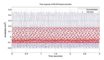
**Figure 22.** Experimental time response of PID-based controller tuned by PSO algorithm. PID: proportional—integral—derivative; PSO: particle swarm optimization.
