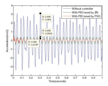
Figure 12. PID controller tuned by ZN and PSO methods for vibration suppression in time domain using multiple sinusoidal disturbance.
