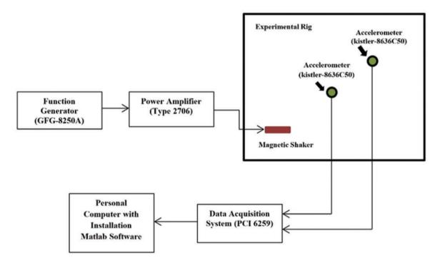
Figure 2. The layout of experimental setup.
