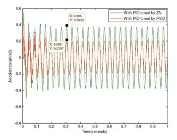
**Figure 14.** Comparison of time domain between PID-ZN controller and PID-ABC controller with multiple sinusoidal disturbance. PID: proportional–integral–derivative; ZN: Ziegler–Nichols; PSO: particle swarm optimization.
