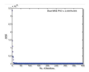
**Figure 3.** Mean square error versus number of generation using particle swarm optimization modeling. MSE: mean squared error; PSO: particle swarm optimization.
