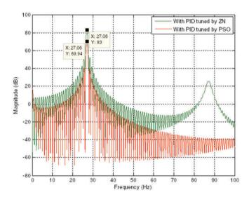
Figure 15. Comparison of frequency domain between PID-ZN controller and PID-ABC controller with multiple sinusoidal disturbance.
