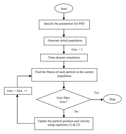
**Figure 11.** The computational flowchart of PSO algorithm. PSO: particle swarm optimization.
