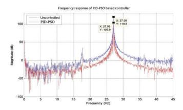
**Figure 23.** Experimental frequency response of PID-based controller tuned by PSO algorithm. PID: proportional–integral–derivative; PSO: particle swarm optimization.
