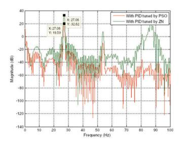
Figure 19. Comparison in frequency domain between PID-ZN controller and PID-ABC controller with multiple real disturbance. PID: proportional—integral—derivative; ZN: Ziegler—Nichols; PSO: particle swarm optimization.
