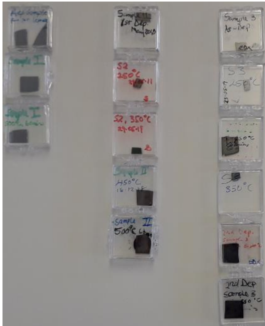
Figure 6.1: The photos of Si substrates for 23% oxygen partial pressure depositions. The samples were labeled S1, S2 and S3 as arranged in the figure. Right on top of the sample I is the Si reference sample.
