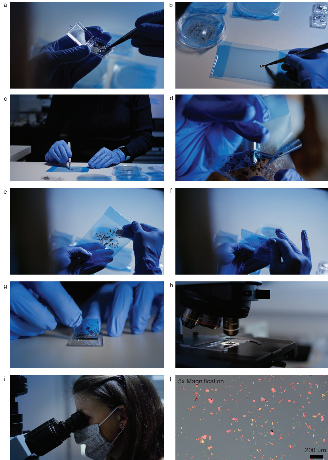
Figure 3.2. Mechanical exfoliation process. Illustration of the technique for exfoliating two-dimensional materials using adhesive tape. The individual steps (a–j) are described in the text (filmstills by schwarzpictures.com).
