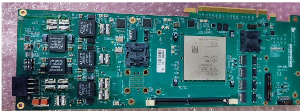
Figure 5.30: Custom board FELIX Phase-II with VU9P.
