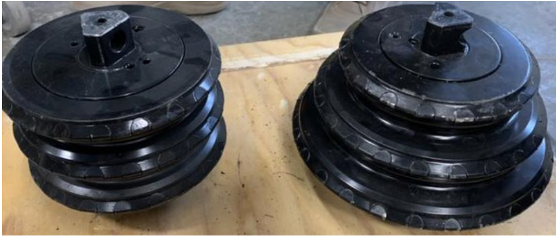
Figure A.1-2 Cylindrical disc cutter (left) and Conical disc cutter (right).
