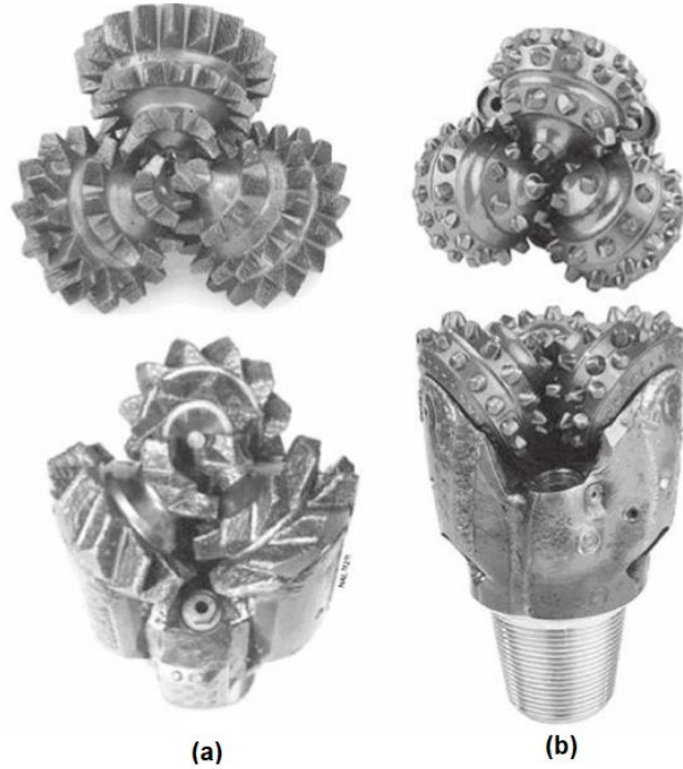
Figure 2-6 (a) Roller-cone milled-tooth and (b) Tungsten carbide insert bits [2].
