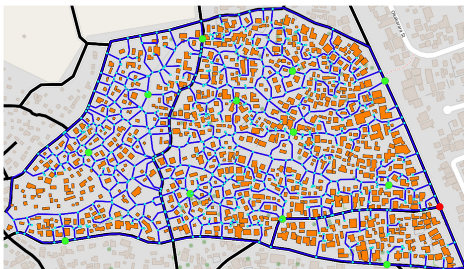
Figure 6. Result of optimal water point-locations (green) in the maximum possible WDS (pipes: blue, nodes: cyan) in the upgrading-area (basemap and buildings/polygons: [36]).
