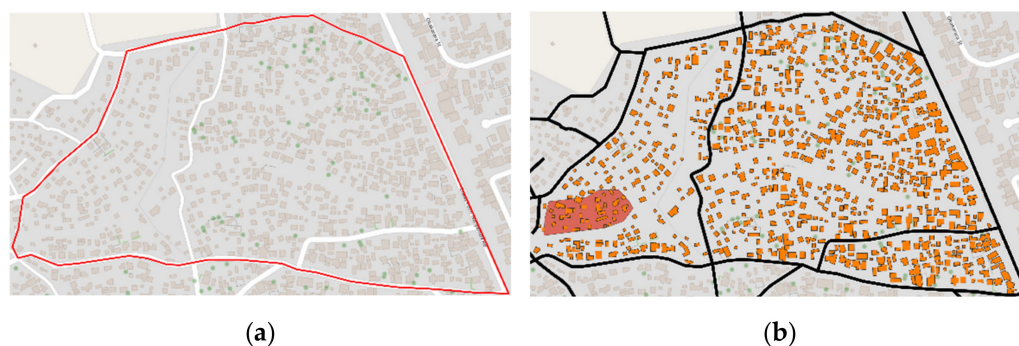
Figure 2. (a) Aerial view of the study area; (b) Method input data from OpenStreetMap [36]: shacks are represented as polygons (orange) and existing paths/roads are represented as line elements (black).
