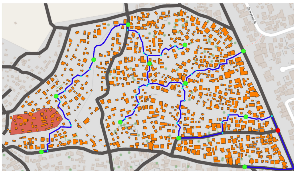
Figure 7. Result of the generated WDS (pipes: blue, water: points green, feeding point: red) without differentiation of ambient conditions (basemap and buildings/polygons: [36]).
