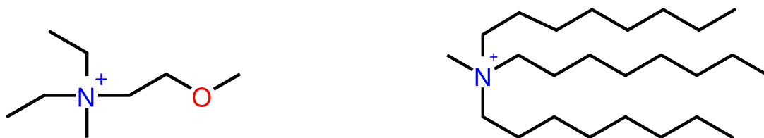
Figure 5.14.: Diethylmethyl(2-methoxyethyl)ammonium [N_{2,2,1,2O1}] on the left and Methyltrioctylammonium [N_{8,8,8,1}] on the right.
