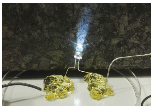
Figure 6.16.: Demonstration of the Ion Jelly mediating charge transfer from a battery to light up a LED.
