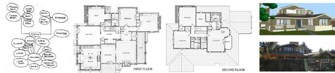
Figure 11.11 – An example of the Program-first approach in real practice. Client requirements are turned into a bubble diagram, which is used to generate a floor plan, which in turn is used to create the 3D model. Image credits: P. Merrell, Schkufza and Koltun 2010.
