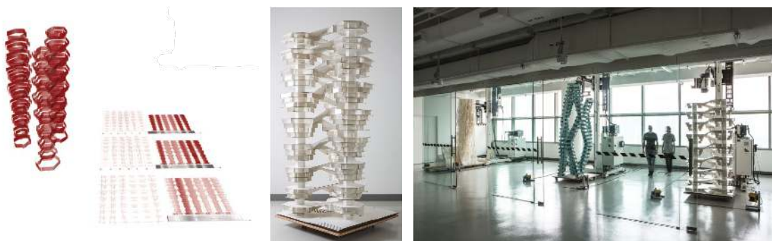
Figure 3.65 – Parametric fabrication-aware scaled model of towers. Left: Parametric model of housing units; Second from left: unfolded wall surfaces; Third from left: the robotically fabricated tower model; Right: the Future Cities Laboratory (FCL) with three robot stations at the Singapore-ETH Centre. Image credits: Budig, Lim and Petrovic 2014.
