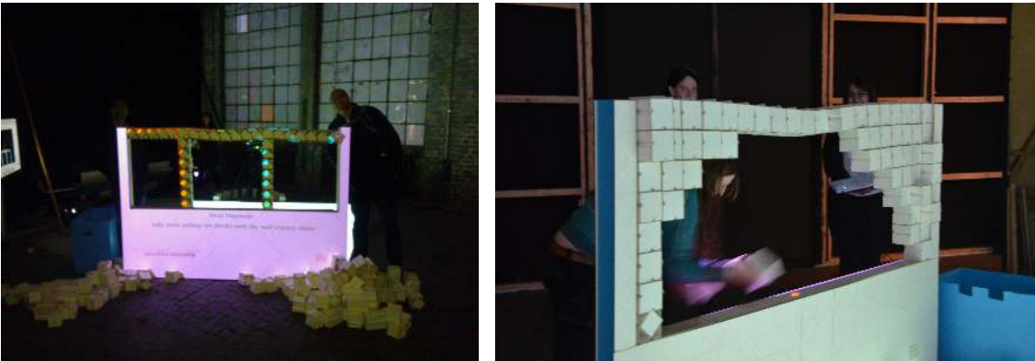
Figure 7.26 – Topological optimization games. Left: An extreme result from a post and beam game type; and right: an 'Arch' game type in progress. Image credits: the author.
