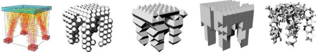
Figure 3.36 – Design interpretations of topologically optimized voxel fields. Using the discrete modeling approach by Rossi and Tessmann 2017a, the same voxel field can have different design expressions. Image credits: Rossi and Tessmann 2017a.
