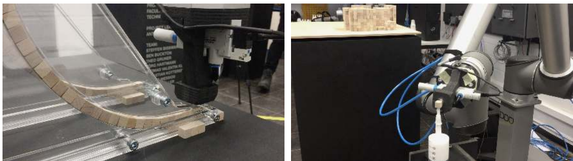
Figure 8.22 – Close-up photos of the robot process components. Left: the robot picking up a cube from the slide of the block dispenser. Right: the robot dipping the cube on the glue-dispensing syringe. Image credits: Rui Nong 2018.
