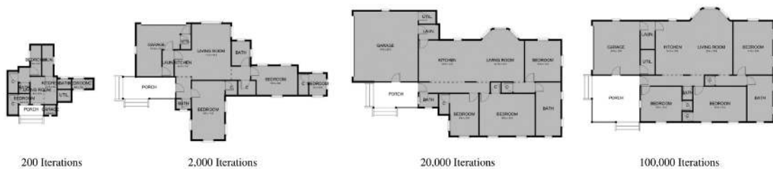
Figure 3.34 – Floor plan optimization using the Metropolis algorithm. Metropolis is a Markov Chain Monte Carlo type of algorithm used in the work of P. Merrell, Schkufza and Koltun 2010. Image credits: P. Merrell, Schkufza and Koltun 2010.
