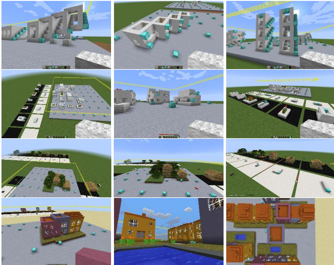
Figure 8.90 – Grammar and vocabulary evolution. Each row shows a selected iteration from the evolution of the shape grammar used in IBA_GAME . Working with generic architectural fragments, shown in the top and the second row, proved too complex for players. The more intuitive approach was to treat elements as means to block out the city's territory (lower two versions). Image credits: the author, Messios, Rudolph.
