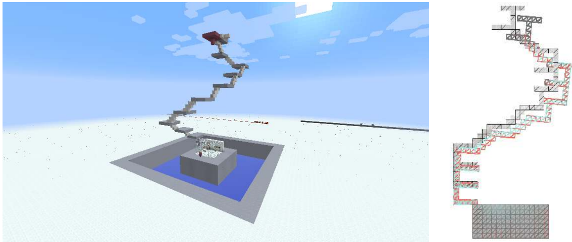
Figure 8.53 – Structural simulation of game results. A player-created structure (left) and its simulated deformation after analysis in Grasshopper with Millipede (right). Image credits: the author.
