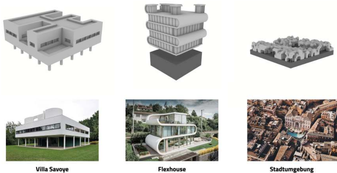
Figure 11.9 – Designs created within Project Reptiles. The generative techniques used here is the iso-surfacing algorithm Marching Cubes. The diversity stems from user-created tilesets. Image credits: the author.
