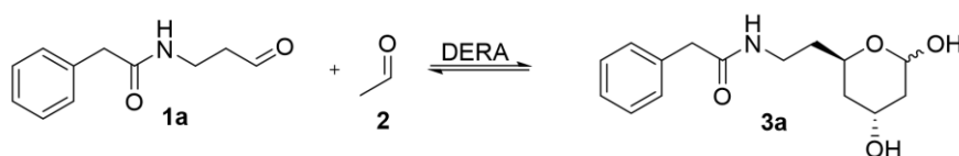
Scheme 3.12 DERA-catalyzed sequential addition of two molecules of acetaldehyde ( 2 ) to PhAc-protected aldehyde 1a .
