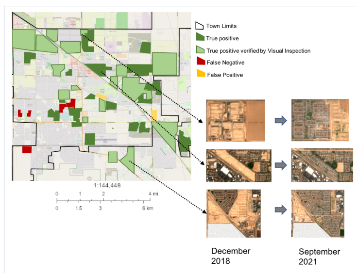
Figure 11. Comparison between change detection results and official documents of Queen Creek Development.
