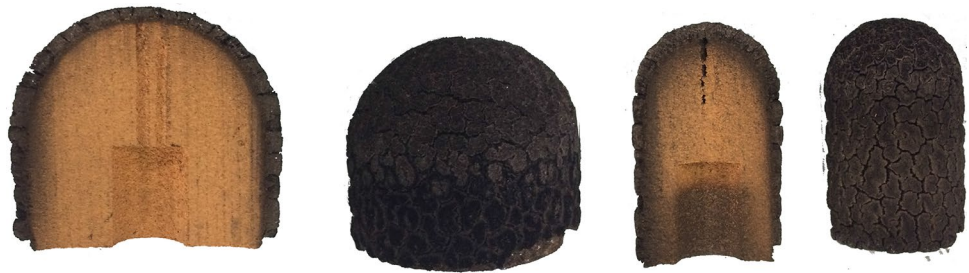
Fig. 8 Cross sections of Tests 14R (left) and 26 (right) with radii of 25 and 15 mm, respectively. 11 mm radius samples were completely charred and could not be removed intact from the sample holder
