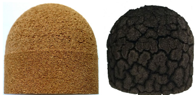
Fig. 7 Change of cork P50 surface topology from virgin (left) to char cracks (right) after Test 9R
