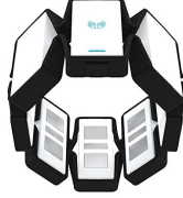
Fig. 9: Myo Armband from Thalmic Labs : an 8-channel EMG sensor used to predict the desired wrist stiffness K_{des} .
