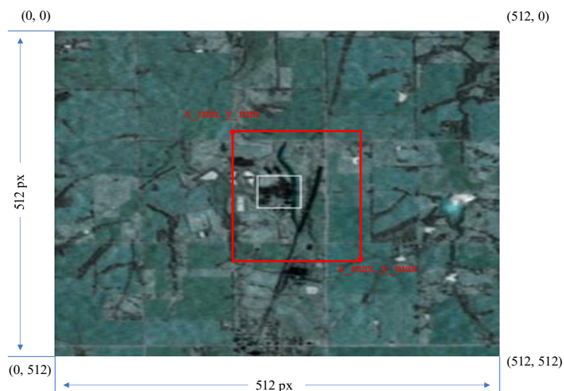
Figure 30. An example image with a bounding box annotation in Pascal VOC format
