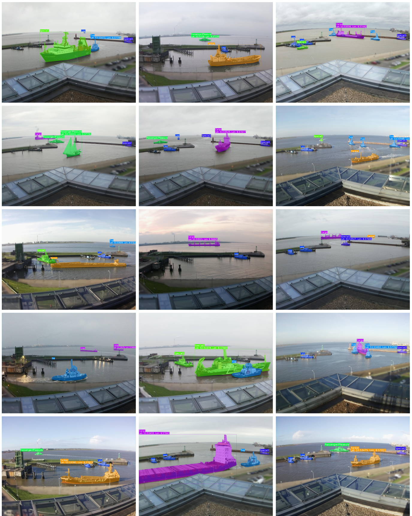
Figure 3. Visualisation of ShipSG dataset samples with annotated ship masks and classes, and one ship position per image.
