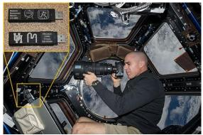
Fig. 2 Space qualified miniaturized Timepix detector (in both yellow boxes) mounted in the cupola of the ISS. These detectors on ESA Proba V satellite are used for years to monitor the dangerous particle radiation in the South Atlantic Anomaly (SAA).
