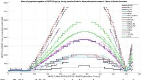
Fig. 7 Plot of PS mass including thruster, redundant PPU and PFS (Propellant Feed System) over mission time of trajectory Earth-Mars featuring relevant thruster types. Breaks show that required thrust is not achieved with this thruster.
