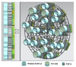
Fig. 6 CAD design of gridded cluster plate including Japanese, Russian and US electric thrusters with redundant PPUs for each thruster at the backside of the INPPS.
