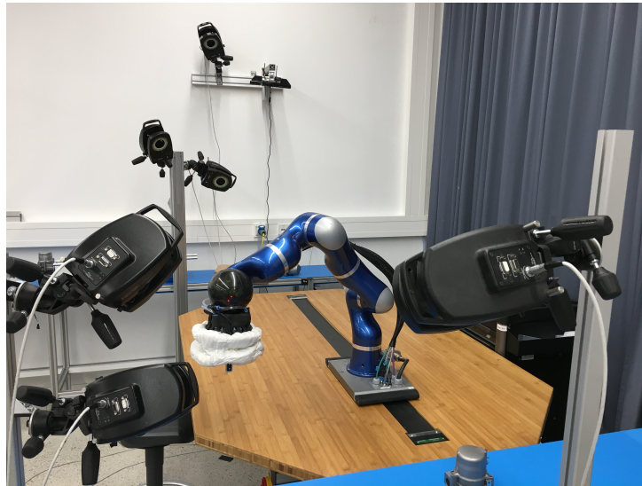
Figure 6.11: The experimental setup on the octagon collaborative workbench is surrounded by VICON marker tracking system to measure the human hand position. Image ©IEEE
