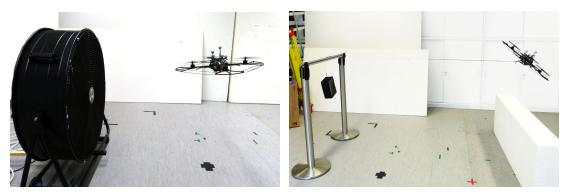
(a) Hovering in a 3 m/s turbulent wind stream, (b) Hovering with a constant side force produced generated by a fan with 70 cm diameter by a suspended 6 N weight
