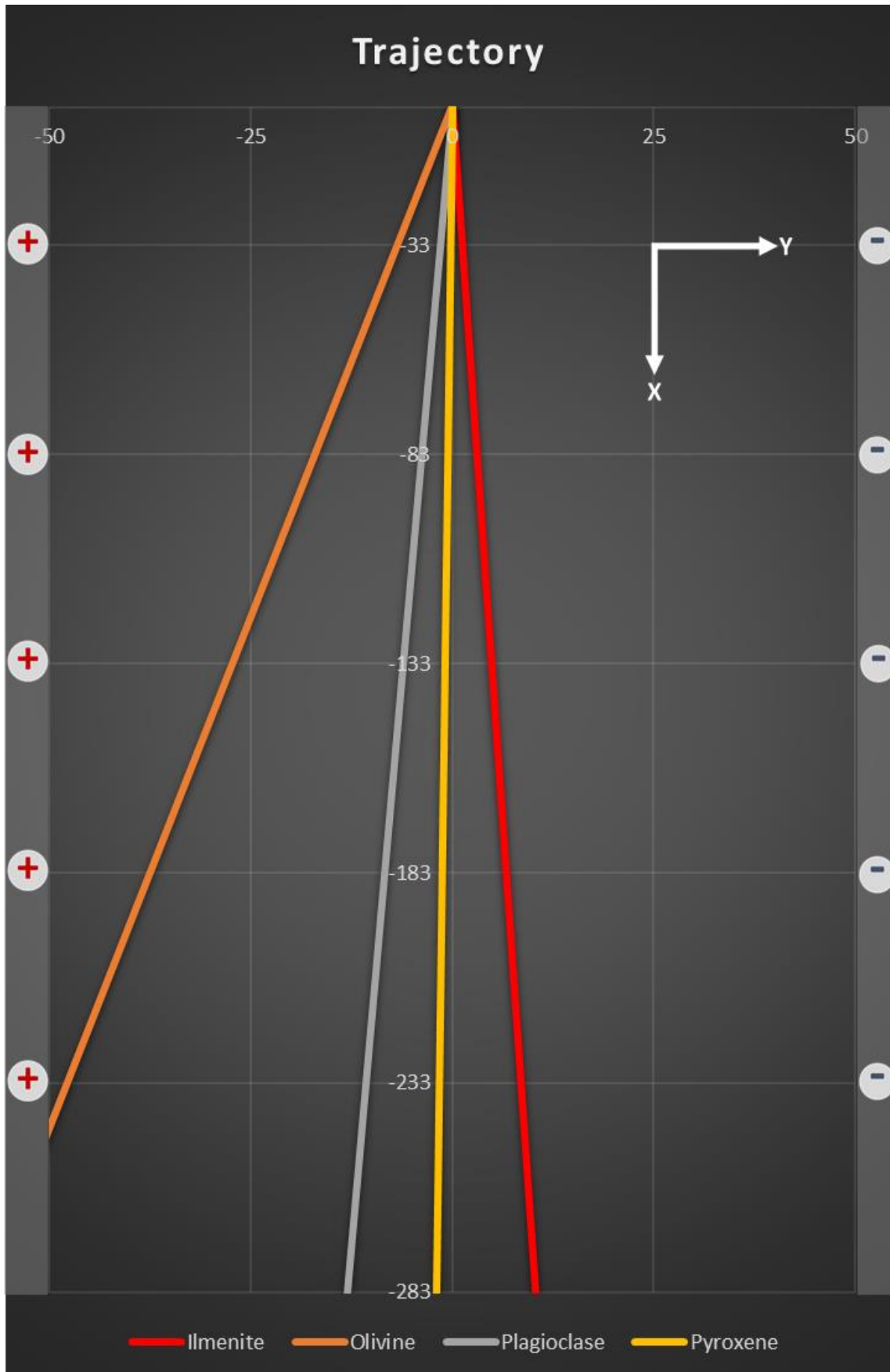
Plot of the Results (using stainless steel chargers on the Moon at 0.5 \cdot U_{max} )
