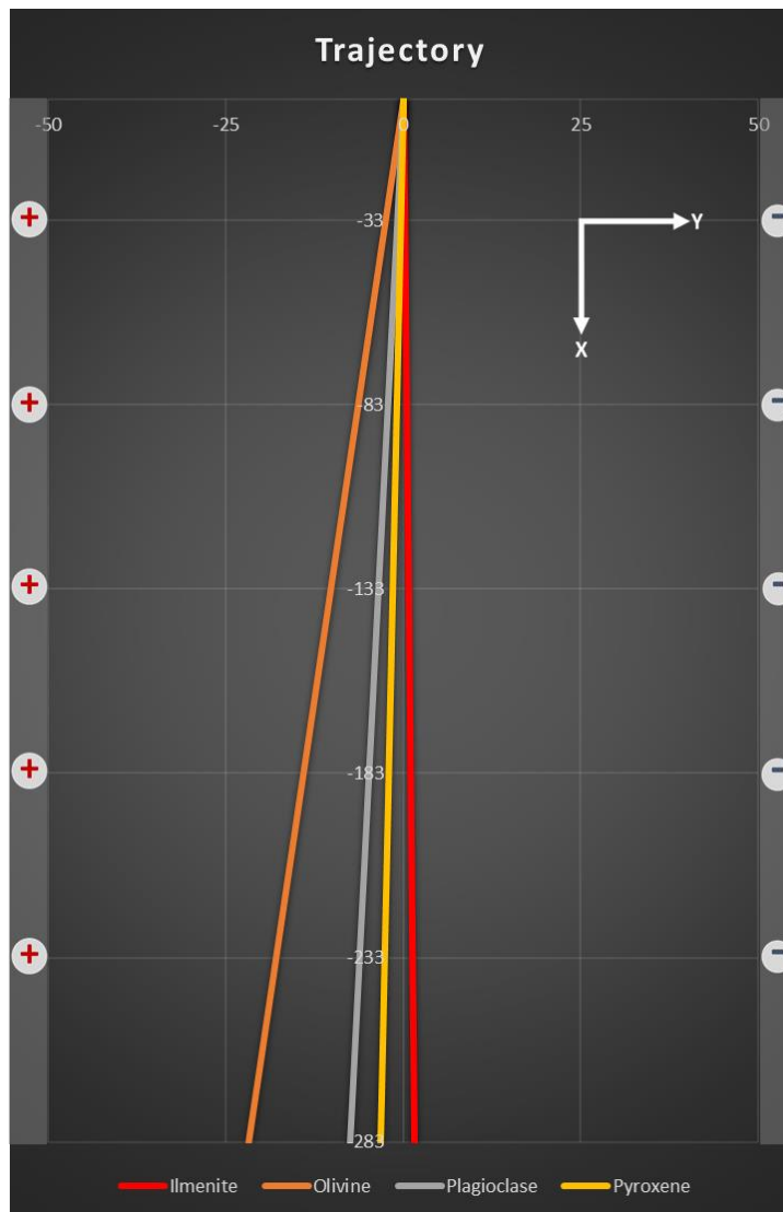
Plot of the Results (using copper chargers on the Earth at U_{max} )
