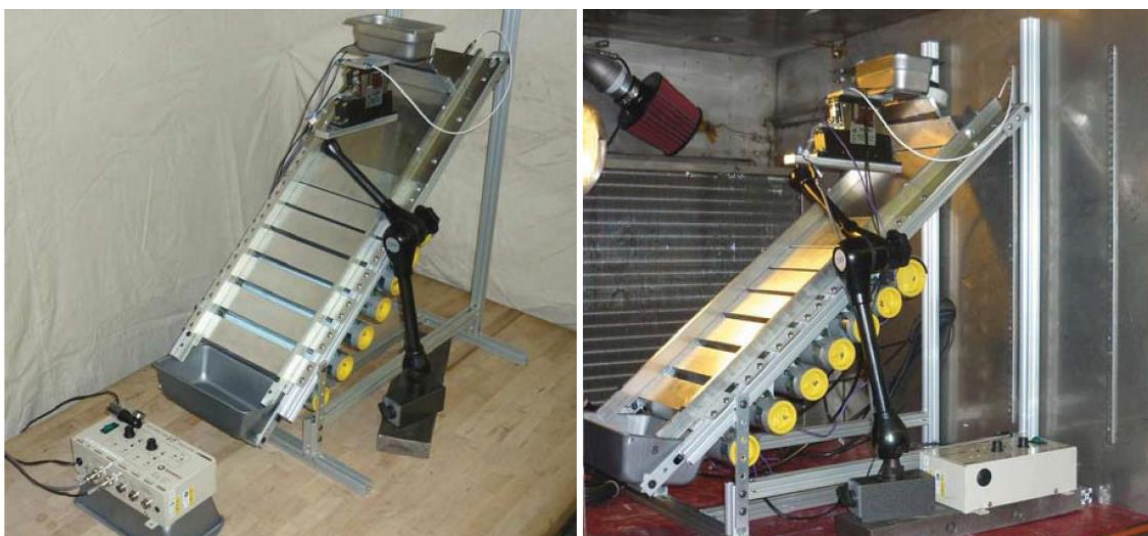
Figure 18: Slotted ramp particle size separator after assembly (L) and in vacuum chamber (R) [20, p. 11]
