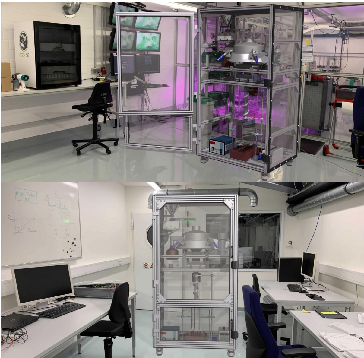
Figure 52: Artistic impressions of SMU's beneficiation test stand inside the laboratory of DLR Bremen
