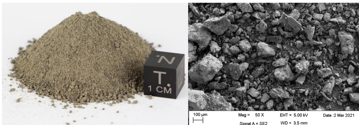
Figure 12: LMS-1 Lunar Mare Simulant appearance and microscopic image [49]
