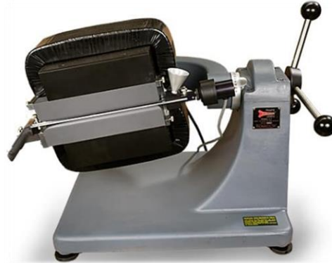
Figure 24: Frantz Isodynamic Separator with external magnet and two-channel track [67]
