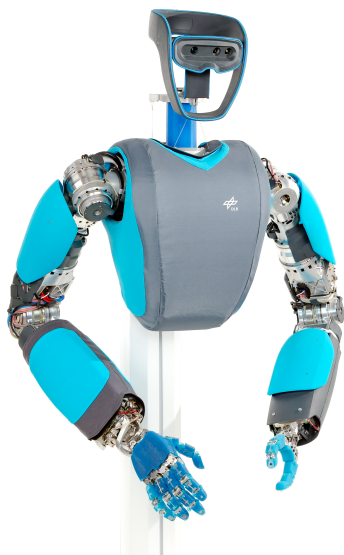
Figure 2.6: The anthropomorphic robot David of DLR using SEA drive concept with an adjustable stiffness and a nonlinear spring characteristic. (Picture by DLR)
