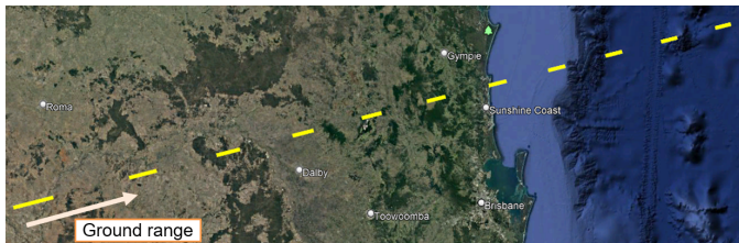
Fig. 2. Illustration of every possible target for a concurrent imaging acquisition over Queensland, Australia, using a PRF of 6088 Hz.
