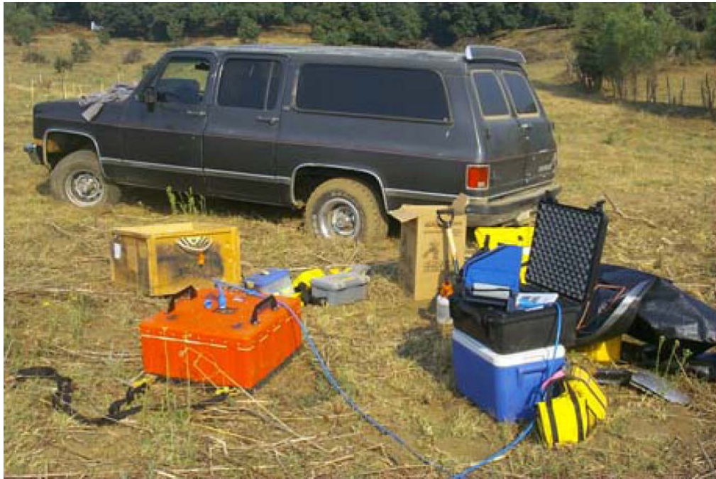
Figure 19. The GSSI SIR 3000 GPR system with the 200 MHz antenna unit at the site.
