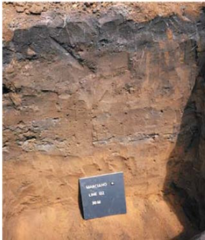
Figure 22. A buried gray consolidated tephra (60-80 cm deep) shown in a 1x2 meter (Liu et al. 2008).
