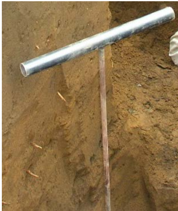
Figure 38. “T” shaped probe used to gather depth data in 2013. The probe was also used to test the bottom of trenches in 2009 as shown in photo.
