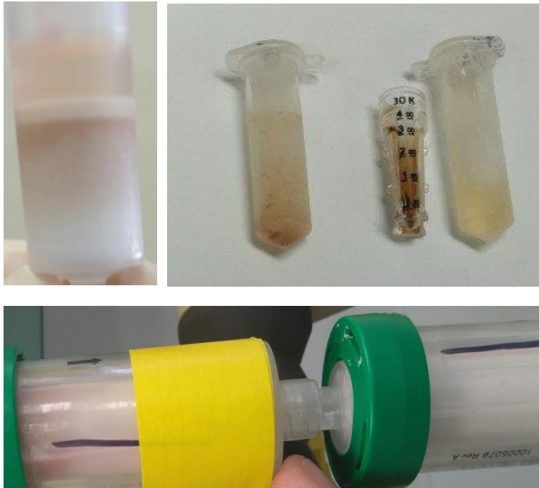
Figure 3.5: Haemoglobin or other ferric contaminants in chromatography. Top left: pinkish-brown pigment binding to SPE column. Top right: B15 before (left) and after (right: insert and outer tube) ultrafiltration through a <30 kDa MWCO membrane. Bottom: Cation exchange columns with pigment (pigment is at the leftwards end).
