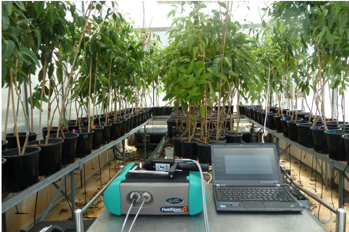
Figure 1. Glasshouse setup during the spectral trials. The ASD FieldSpec spectrometer was setup in front of the glasshouse. The Corymbia calophylla plants were carried to the spectrometer, and the measurements taken by clipping the leaf probe onto the youngest, fully expanded leaf.
