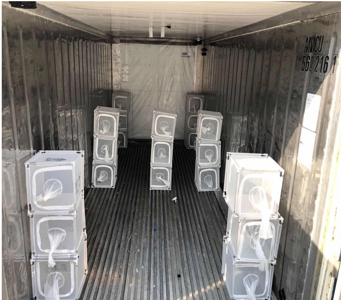
Figure 3-4. Insect cages within shipping container used for commercial fumigation trials.
