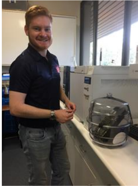
Figure 5-3. Conducting fumigation of graphics processing unit using desiccator (9.9 L) as the fumigation chamber with ethyl formate and methyl bromide.
