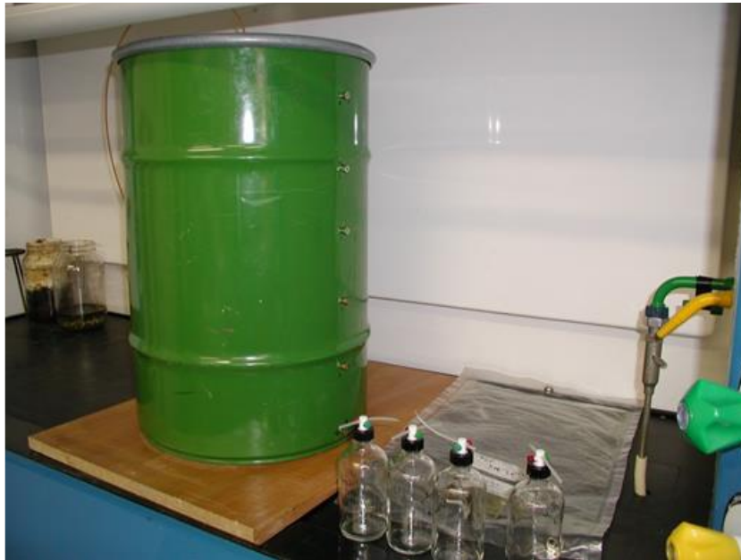
Figure 5-2. The fumigation chamber (60 L) used for preliminary investigation of ethyl formate inter reaction with materials, equipped with gas injection and sampling systems.
