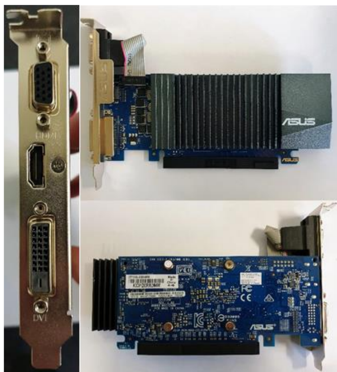
Figure 5-1. Graphics processing unit selected for fumigation with ethyl formate and methyl bromide.
