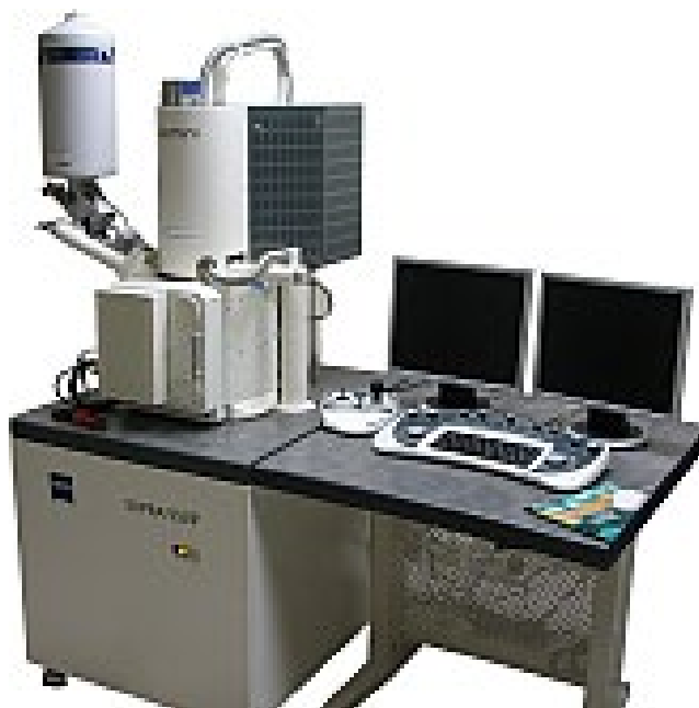
Figure 3.1. High-resolution scanning electron microscope (SEM) Zeiss 55 VP-SEM used for scanning the SAS treated adult R. dominica .
