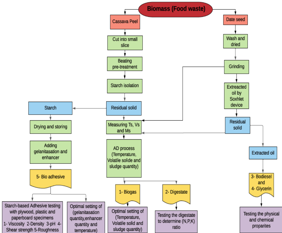
Figure 28: The experimental procedure flowchart.
