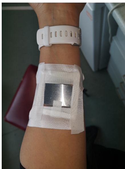
Figure 3.6 Image showing the MAP sensor as worn on the skin in the participant study.
