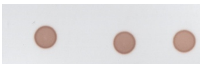
Figure 3.15 Drop-cast MAP dye (1 \mu L) from a 20 mM THF solution on silica TLC paper. Note: Image is following exposure to ammonia (30 ppm).
