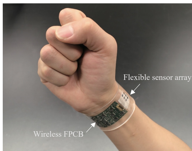
Figure 1.4 Photograph of the wearable sensor on a subjects wrist showing the flexible sensor array and wireless FPCB developed by Gao et al. 96
