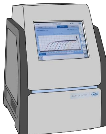
Figure 3. 23. Schematic representation of the LightCycler ® 96 Instrument, Roche
