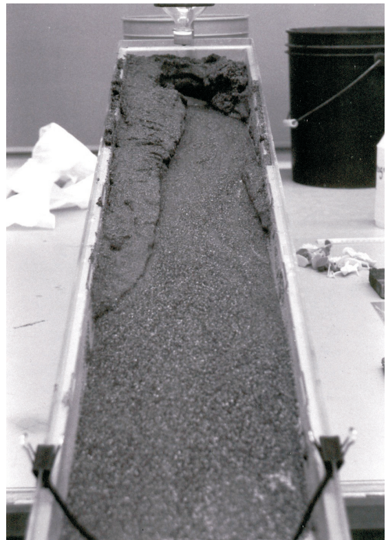
Figure 4. Effects of low (4a) and high (4b) slope angles. Note the differing degrees of incision, braiding, and fan-delta deposition.
