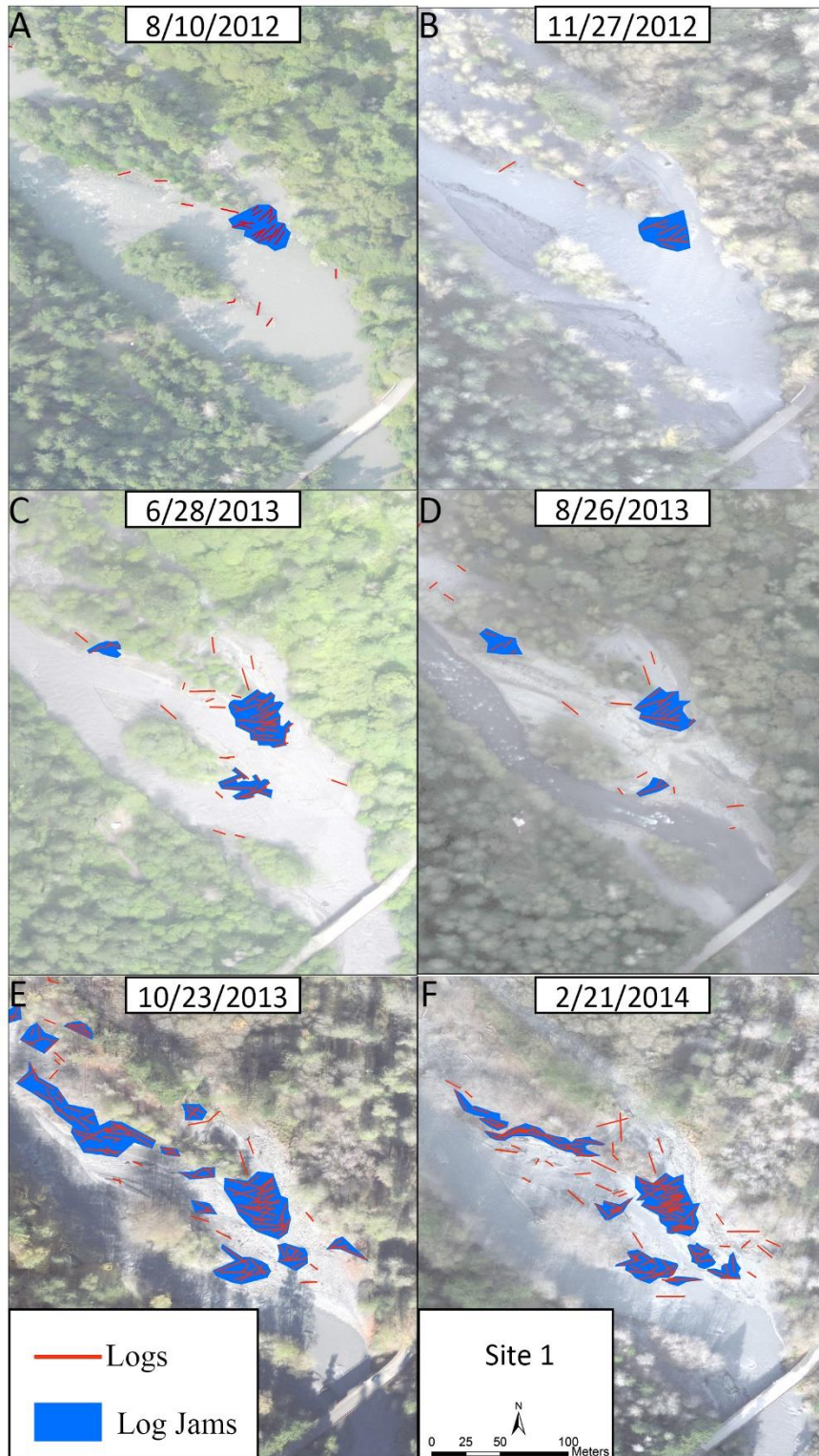
Figure 20: Site 1, Mapping showing the flux of woody debris at the survey site on orthophotographs taken from August 2012-February 2014. Blue = Log Jam Red = Individual logs >2 m in length.
