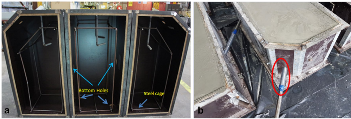
Fig. 5 a structure of reinforced casting mould for 45° cable bolt inclination. b Concrete cast in the mould
