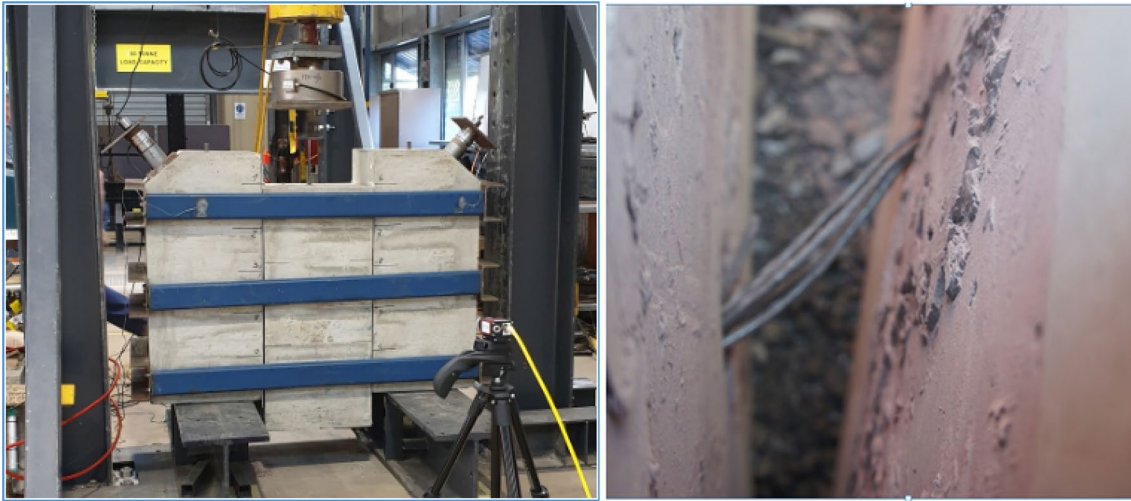
Fig. 13 Centre block shear displacement in which both cable have failed symmetrically. Note the snapped and smeared leaked grout between concrete joint faces
