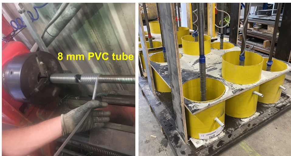
Fig. 4 Preparation of the cylindrical concrete blocks and casting of rifled holes in concrete block using PVC flexible tubes wrapped around the central steel rod
