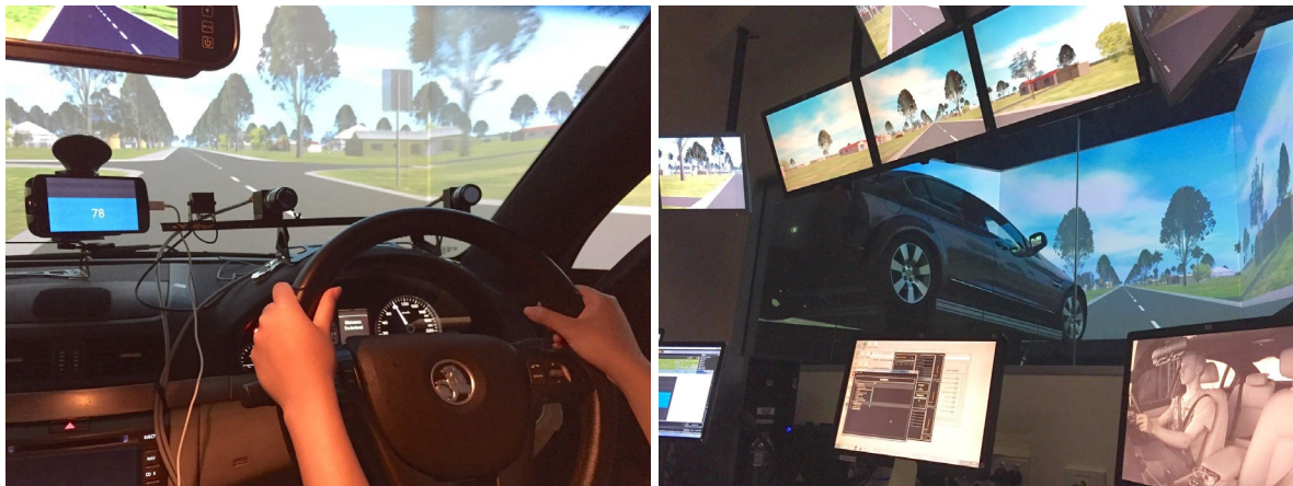
Figure 1: The driving simulator from a participant's perspective (left) and from within the researchers' control room (right).
