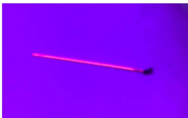
Figure E.6. Photograph of ammonothermally synthesized red luminescence \text{Sr}_3\text{P}_3\text{N}_7:\text{Eu}^{2+} powder in a glass capillary when irradiated with UV light.
