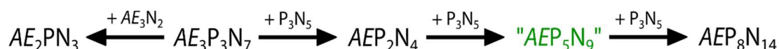
Figure 11.2. Overview of known ternary alkaline earth metal nitridophosphates. Compositional relations of adjacent compounds are indicated by the formal addition of P_3N_5 or AE_3N_2 . Hypothetical “ AEP_5N_9 ” (green) is indicated as stoichiometric void between AEP_2N_4 and AEP_8N_{14} .
