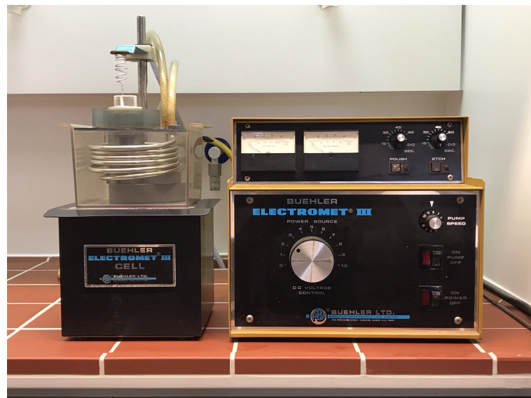
Figure B.1: “Electromet III” with customized sample holder used for electropolishing of aluminum microsections.
