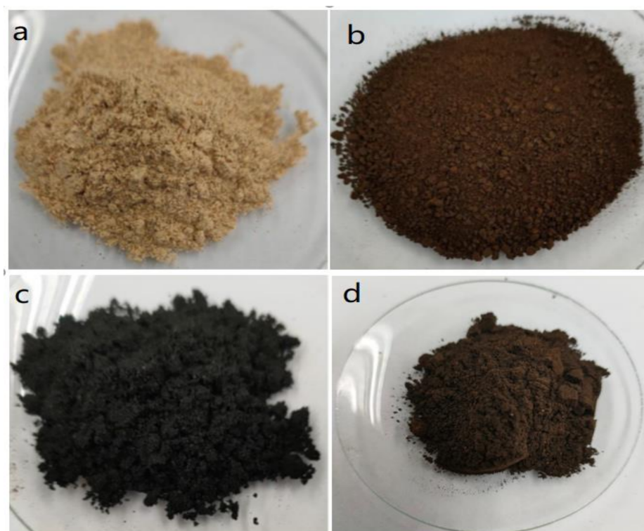
Figure 4. Photographic images for (a) Feedstock, (b) HTC180, (c) PY500, and (d) MW300.
