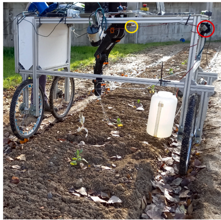
(a) Robotic platform in a small cabbage row. The RGB camera is shown marked in red and the multi-spectral camera in yellow
