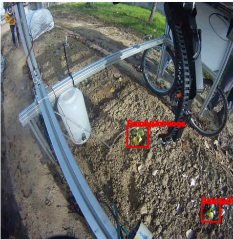
(c) Treatment application with the robot arm to the central small cabbage.
