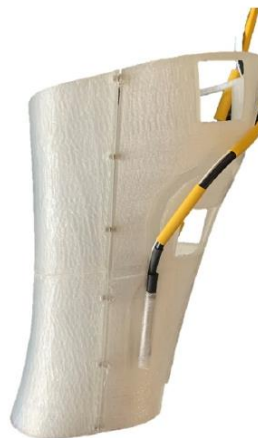
Figure 10: Real model of the splint assembled with the sensors electronic board
