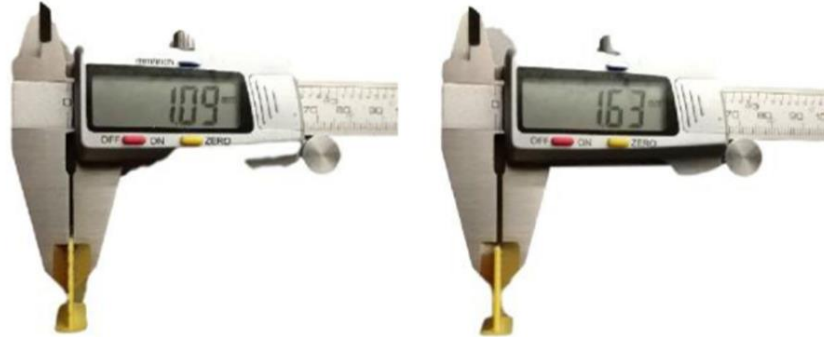
Fig. 2 Error due to filament diameter variations
