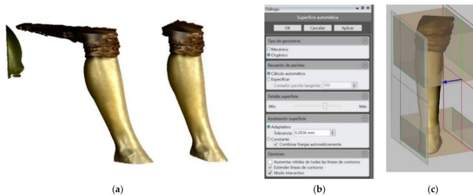
Figure 3. (a) Original and treated points cloud in Geomagic Software; (b) Mesh surface creation parameters; (c) Mesh manipulation.
