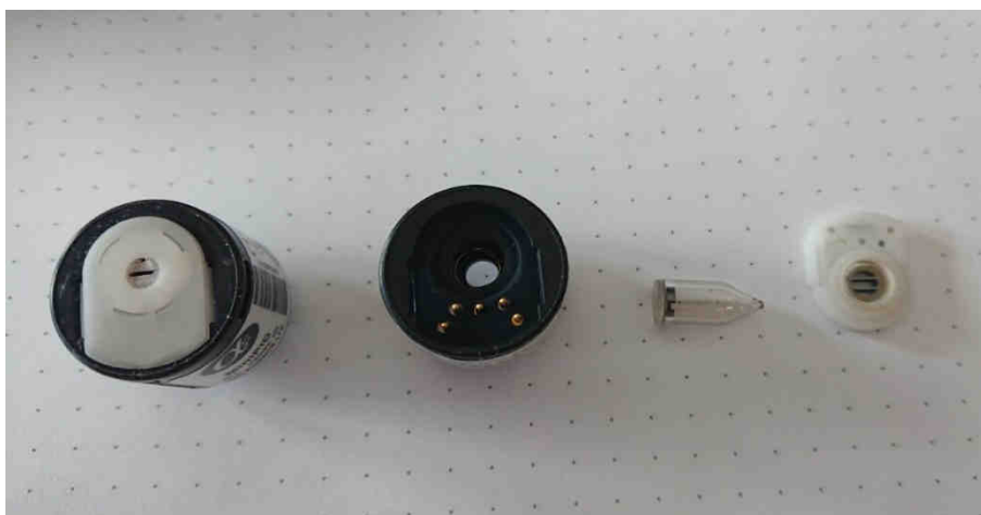
Fig. 3. Alphasense photoionisation sensor; Left to right: completed sensor, sensor body with electronics and contacts, discharge lamp and measuring cell with visible electrodes; Background point pitch 5 mm
