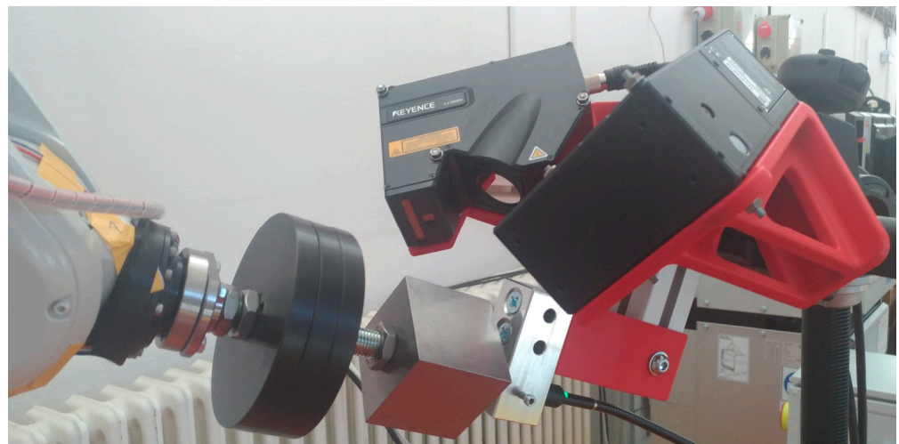
Figure 4. Measuring nest. A robot with the payload tool approaches to confocal sensor that measures the TCP Z-axis distance. TCP X and Y are measured by a pair of laser profilers above the payload tool.
