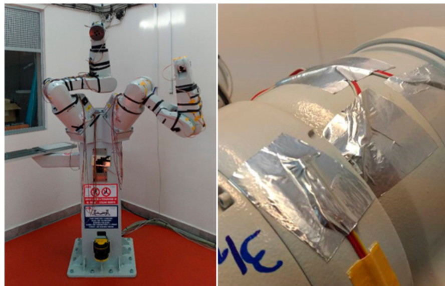
Figure 1. Thermal sensors, in detail on the second joint of the IRB1200 robot.
