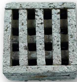
Figure 16. Detail of the casting after removal of the gating system.
