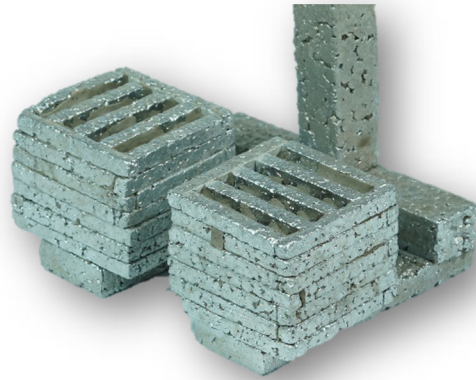
Figure 15. Final pair of castings with gating system after removal from the mould and cleaning.
