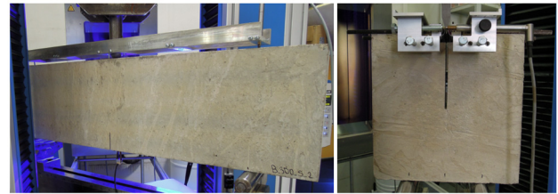
Fig. 2: Test configurations of a three-point bending test (left) and wedge-splitting test (right).
