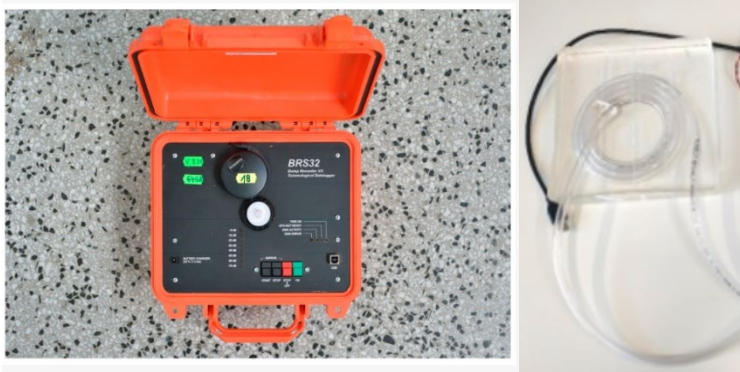
Fig. 1. Reference seismograph BRS32 (left) and tested pneumatic sensor (right).
