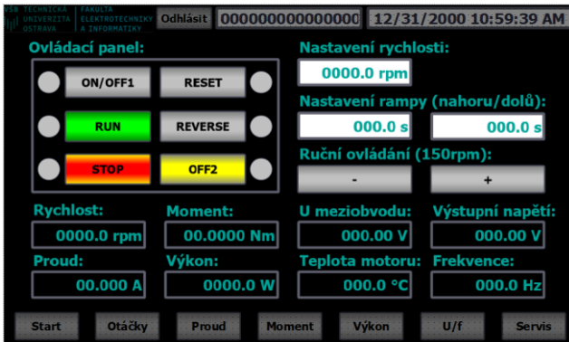
Fig. 3. Preview of the SCADA visualization on HMI panel
