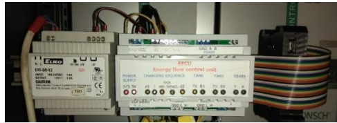
Fig. 3. Hardware realization of the EFCU
