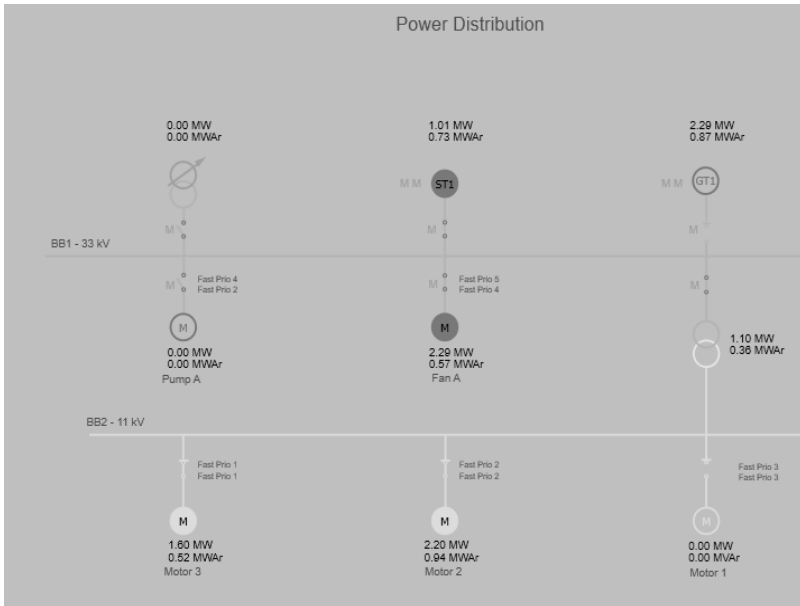
Fig. 4. Graphical display for substation control
