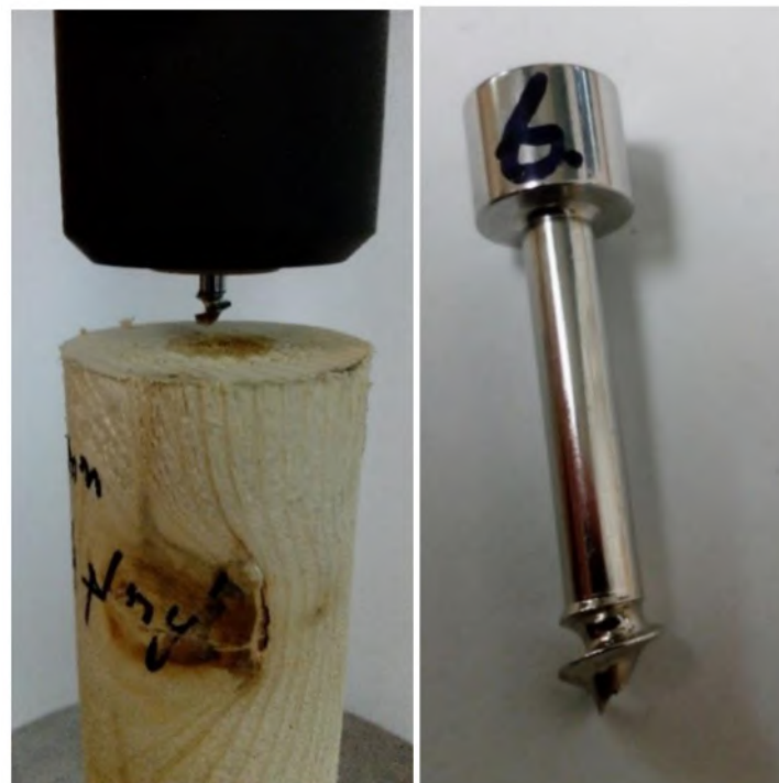
Figure 7. Pull-out test, measurement No. 6 (screw breakage, end of measurement).
