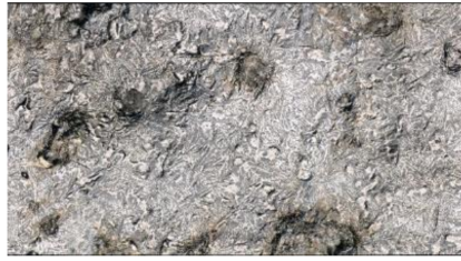
Figure 11. Surface quality W303, magnification 500×.
