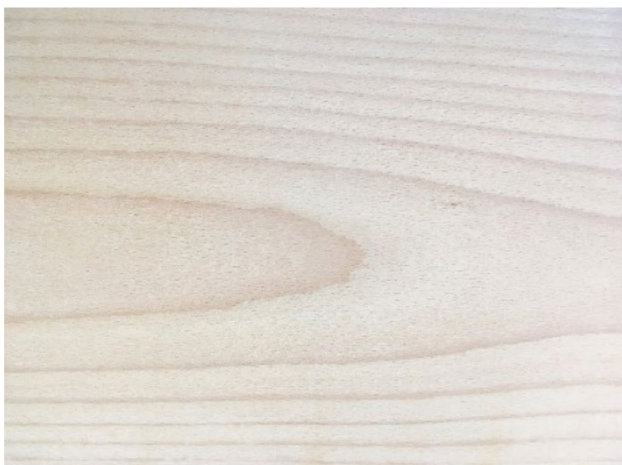
Fig. 2 Beech veneer sample
